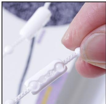
To fit the chain break connectors, join the control chain by placing the last ball of each end of the chain into the larger holes on each side of the connector. If your chain is a continuous loop, close your blind fully and cut the loop on the side nearest the window at the top of the blind for standard roll, or the front of loop if reverse roll. Next, measure 20cm down the chain and cut it at the nearest ball. Then join the chain with a second chain break connector in the same way as above.
