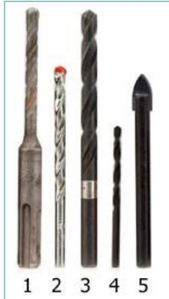
tile only, then change to the Ø5.5mm masonry Drill Bit (fig 2,1) to drill the remainder of the hole. Use Red Rawlplug (fig 6) or Fisher Plaster Plug (fig 7) dependant on your lintel type i.e. concrete, metal or is it hollow? Use the same method as described above for fixings, the Ø8mm larger hole in the tile will prevent the tile cracking when the Rawlplug expands with the screws.
